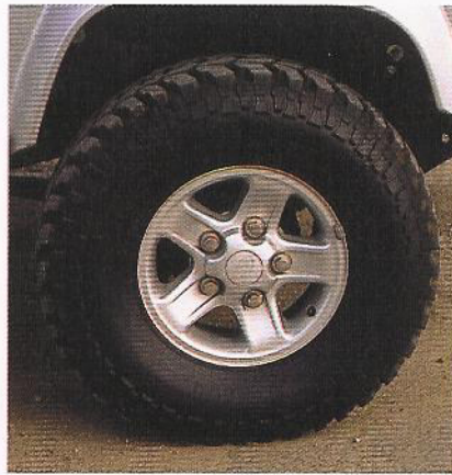
Wheels are new OE Defender 110 rolling stock, wrapped by P285/75R16 Firestone Destination mud-terrains.
