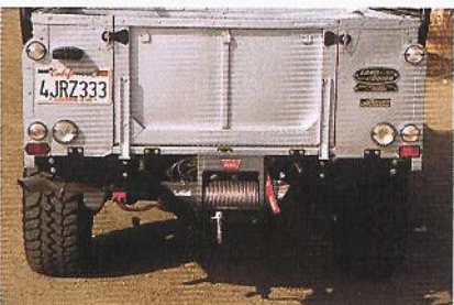
There is a second Warn winch mounted on the rear bumper.
